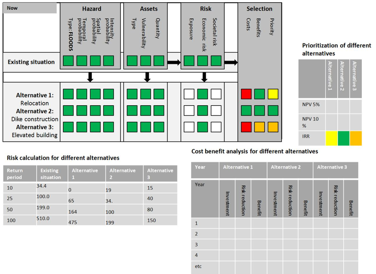
**Figure 4** after analysing the risk after implementing the alternatives, the user can analyse the costs of the alternatives, and make a cost-benefit analysis, leading to a prioritization of the alternatives
