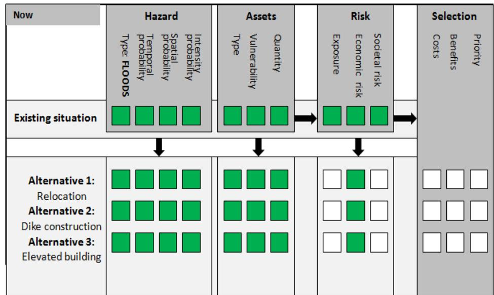
Figure 3 after entering the relevant hazard, assets and vulnerability data for each scenario, the user can analyse the new risk level. He can choose to do it for different types of risk
