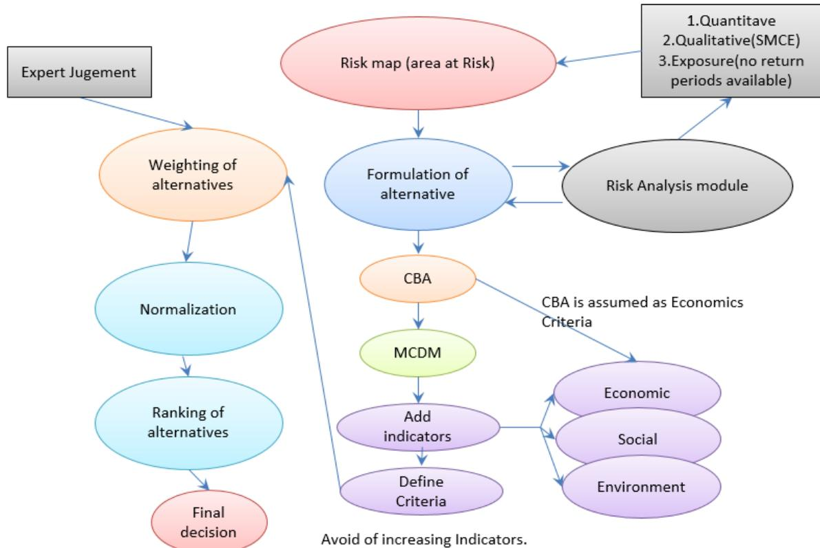
**Figure 5 flowchart of MCDM: After analysing the risk after implementing the alternatives, the user can analyse the costs of the alternatives, and make a cost-benefit analysis, leading to a prioritization of the alternatives**
