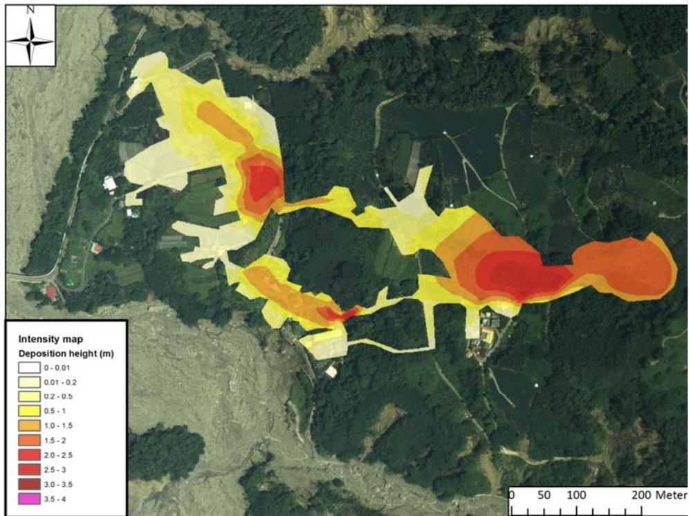
Figure 3: Intensity map of the DF055 in Lai-Ji based on photographic event documentation (Fischer 2014).
