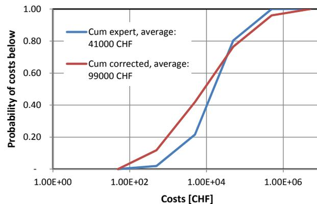
Figure 7: curve of exceedance using the limit of the classes for both corrected and uncorrected probabilities.
