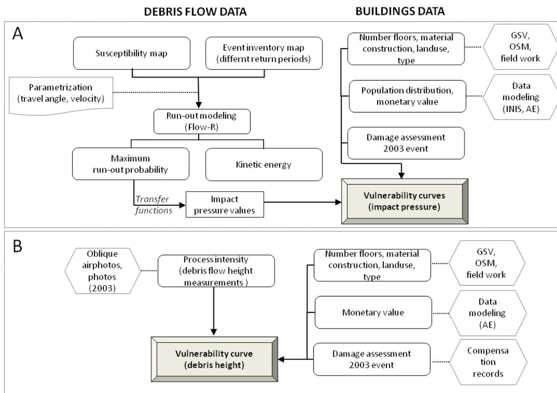
Figure 2. Methodological steps used for vulnerability assessment of buildings to debris-flows in Fella River Basin (A - regional scale: using dynamic run-out modeling; B – local scale: using photo-documentation)
