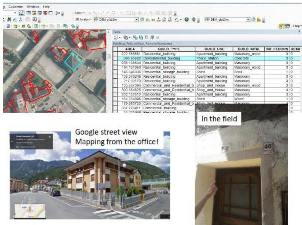
Figure 3. Update and validation of building inventory using Google Street View and field work
