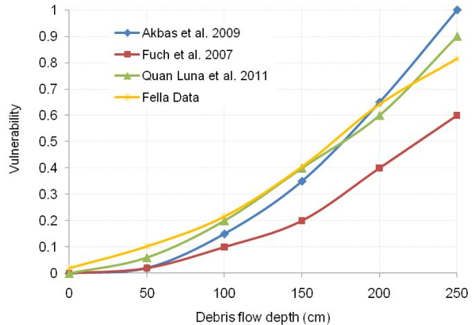
Figure 5. Debris flow vulnerability curve for debris height (Fella Data) in comparison with results from other similar case studies
