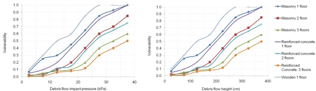
Figure 4. Debris flow vulnerability curves for impact pressure (left) and debris height (right)
