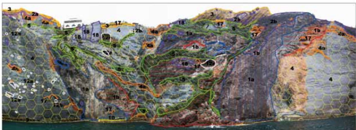
Fig. 7. Geomorphological photo-mosaic map at Cala Inferno. Key: 1) columnar-jointed (a – M1a) or cataclasized (b – M1b) rhyolitic cliff; 2) hyaloclastic rock slope with medium-high gradient covered by soils in accelerated erosion (a – M2a) or with vegetation (b – M2b); 3) cantilever rock slope sector ( H/L \ll 1 – M3); 4) hyaloclastic cliff (a – M4a), with overhanging sectors (b – M4b); 5) rock slope with medium-low gradient covered by detrital and eluvial-colluvial deposits (M5); 10) beach (M11); 12) erosional (a – M10) or anthropogenic (b – M10) cavities; 17) landslides crown (M9); 18) slope sector with unstable rock blocks (M8).
