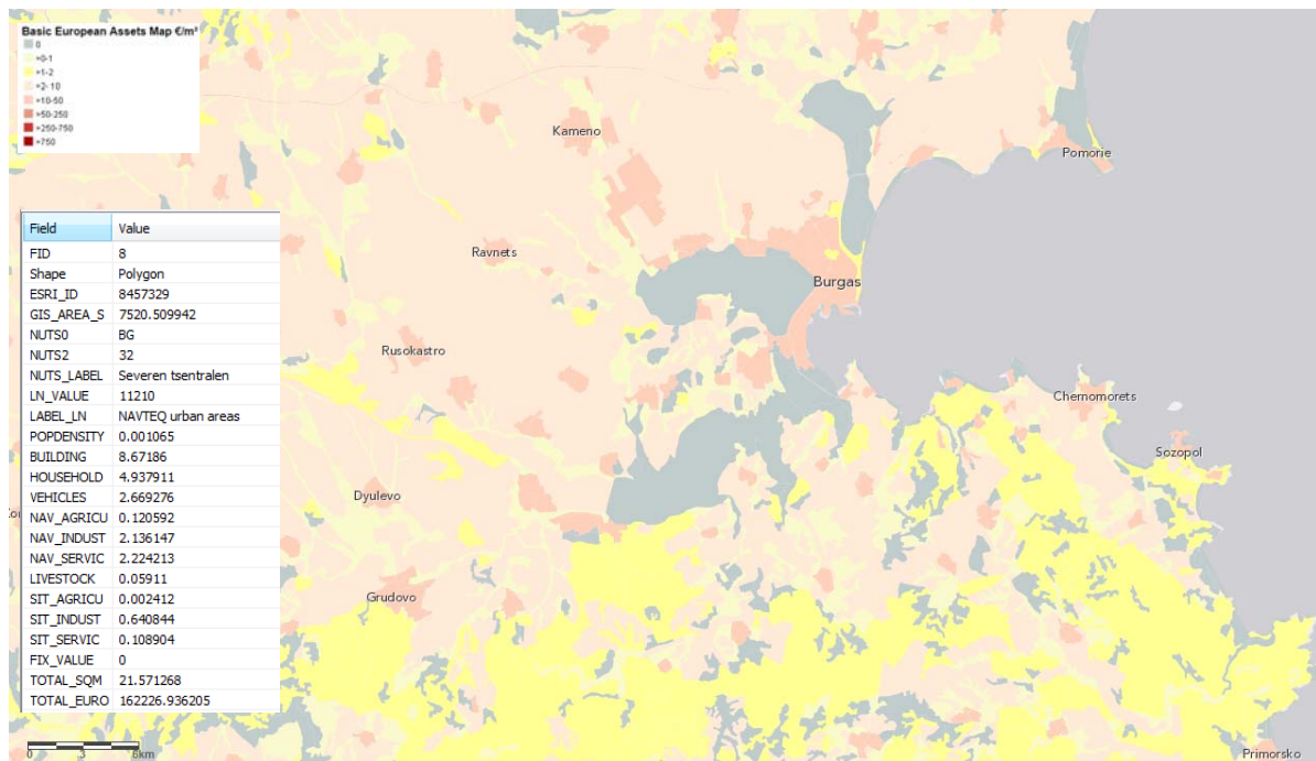
Figure 6: Example of BEAM layer for the coastline of Bulgaria. BEAM contains asset values for buildings, household, vehicles, livestock, both net asset values and stock in trade values of agriculture, industry and service and trade, and more. Source: geomer GmbH.
