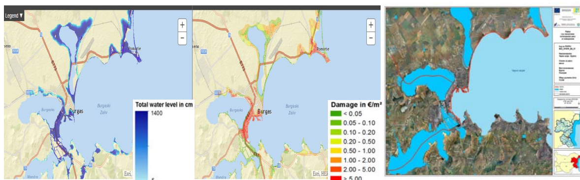
Figure 5: Flood hazard map (left) and risk map (middle) for the Bulgarian coast of the Black sea (area near the town of Pomorie) and schematic map of end-user (right). Source: geomer GmbH & BDBS.
