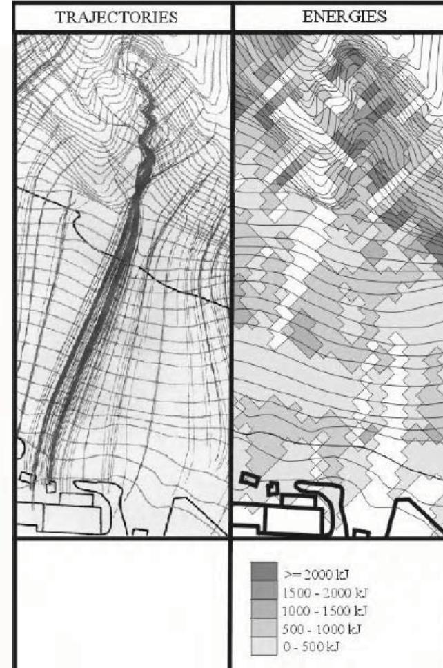
Design of remedial and protective measures are based on landslide intensity calculations !
