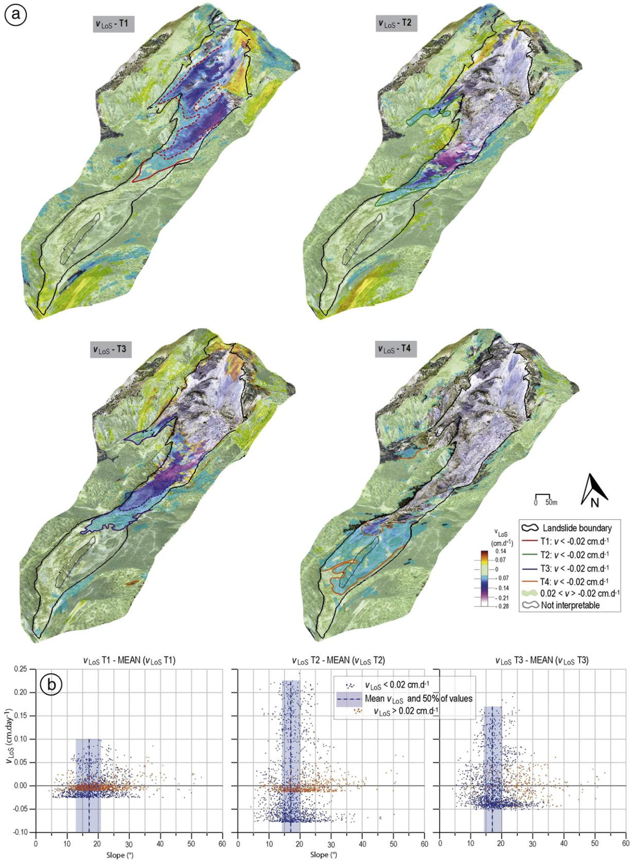
**Fig. 14.** InSAR displacement rates of the La Valette landslide for three periods in 2007 and 2009. (a) Maps of  $v_{LoS}$  values (cm day<sup>-1</sup>) at T1, T2, T3 and T4; (b) plots of  $v_{LoS}$  values as a function of slope angle (°). The velocity estimated at one pixel location is represented in relation to the average velocity observed in the subsidence zone ( $v_{LoS} > 0.02$  cm d<sup>-1</sup>, in orange) and in the transit zone ( $v_{LoS} < 0.02$  cm d<sup>-1</sup>, in blue).
