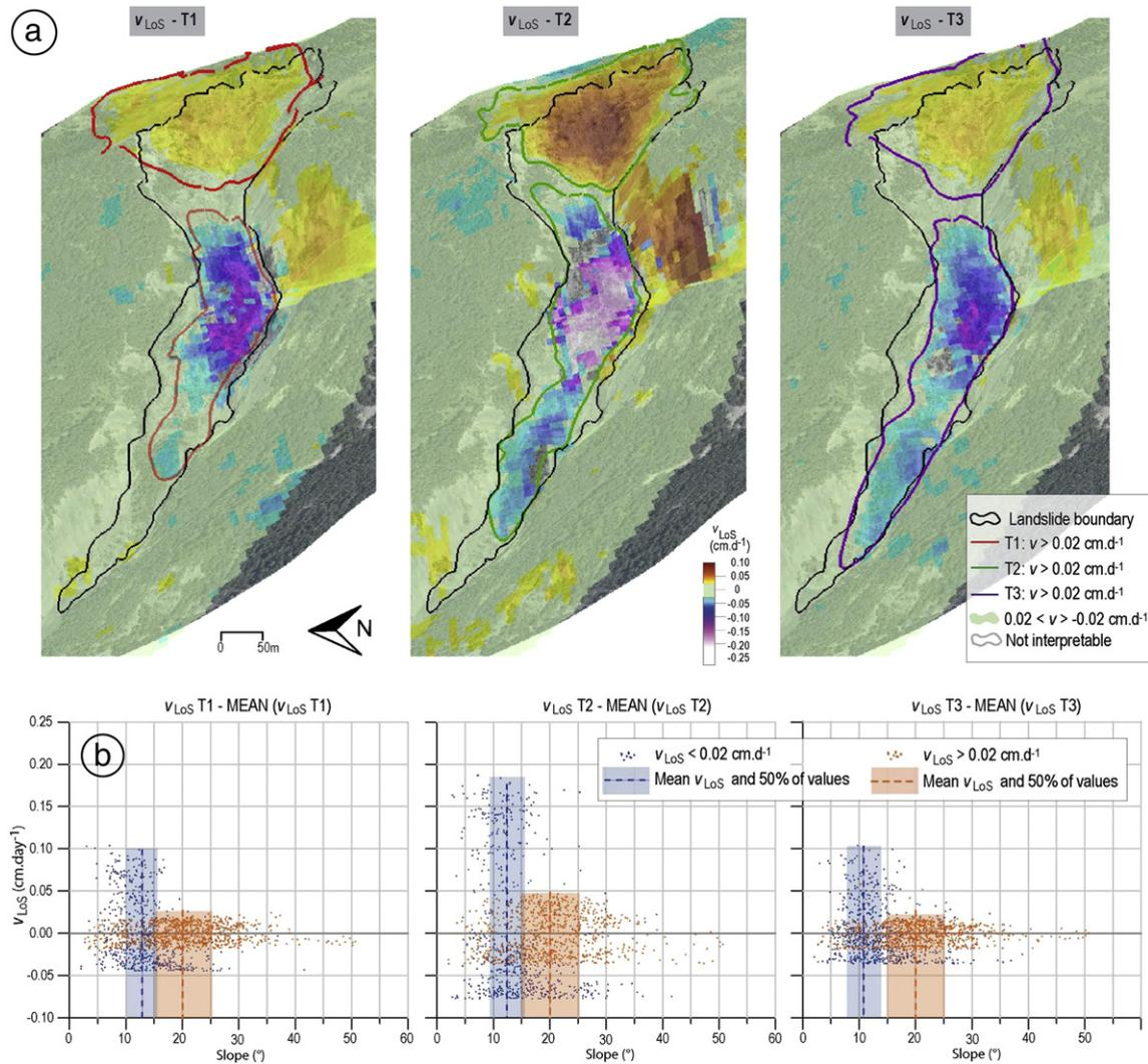
**Fig. 13.** InSAR displacement rates of the Poche landslide for three periods in 2007 and 2009. (a) Maps of  $v_{LoS}$  values ( $cm\ day^{-1}$ ) at T1, T2 and T3. (b) Plots of  $v_{LoS}$  values as a function of slope angle ( $^{\circ}$ ). The velocity estimated at one pixel location is represented in relation to the average velocity observed in the subsidence zone ( $v_{LoS} > 0.02\ cm\ d^{-1}$ , in orange) and in the transit zone ( $v_{LoS} < 0.02\ cm\ d^{-1}$ , in blue).
