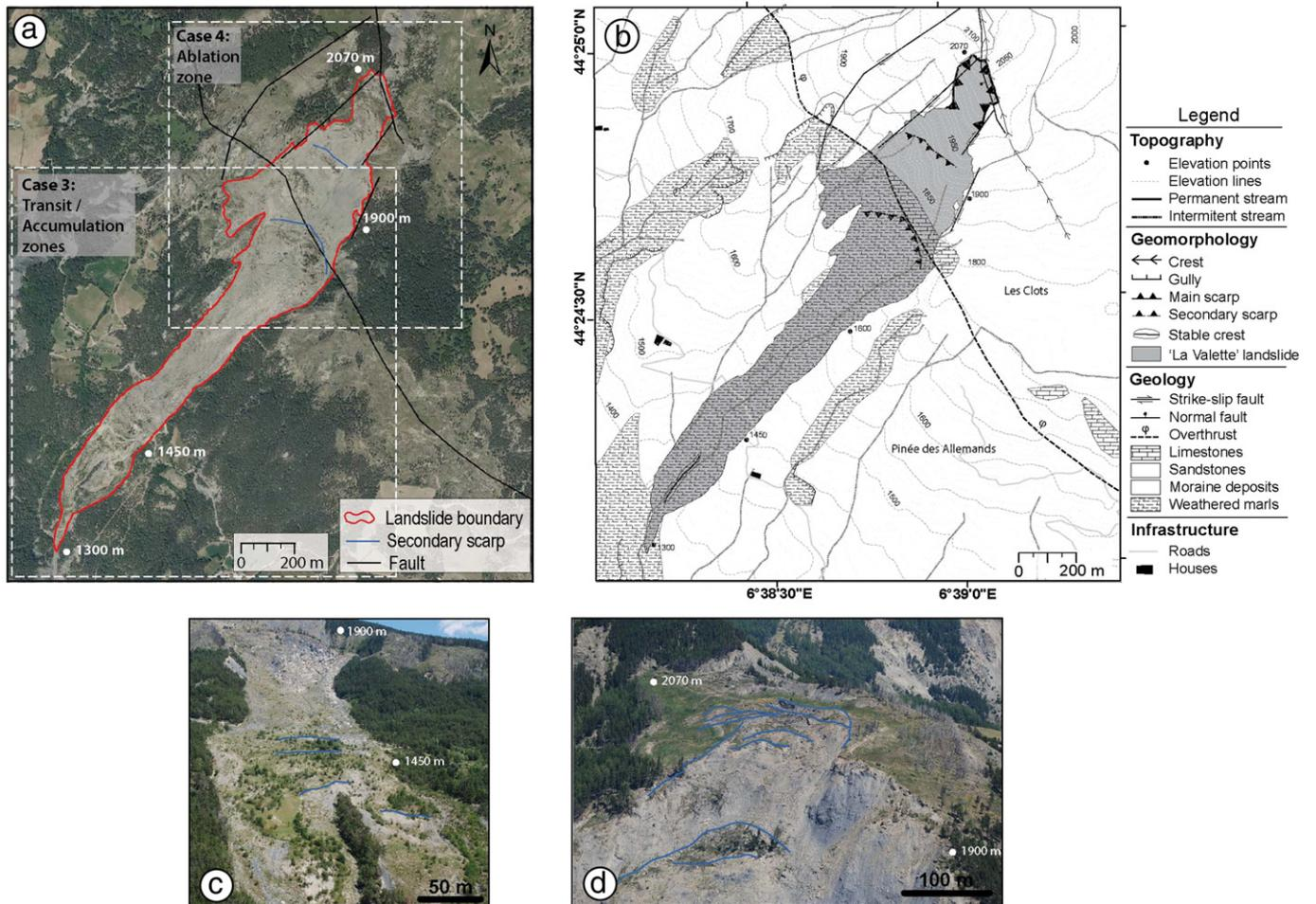
**Fig. 4.** Morphology of the La Valette landslide. (a) Orthophotograph of the landslide in 2009 and location of ablation (case 4) and transit-accumulation zones (case 3), (b) morpho-structural map of the landslide. (c) Photograph of the transit and accumulation zones in 2009. (d) Photograph of the ablation zone in 2009 including numerous secondary scarps.
