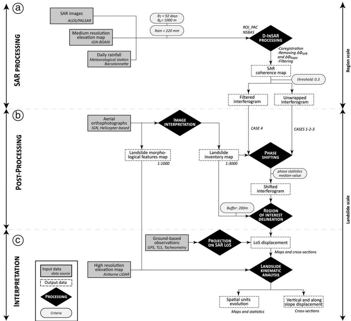
**Fig. 5.** Methodological flowchart and indications of the data and outputs used at each processing step. (a) SAR images selection and processing. (b) Interferograms post-processing. (c) Interferograms interpretation. The detailed characteristics of the data are presented in Table 3 and Fig. 6.
