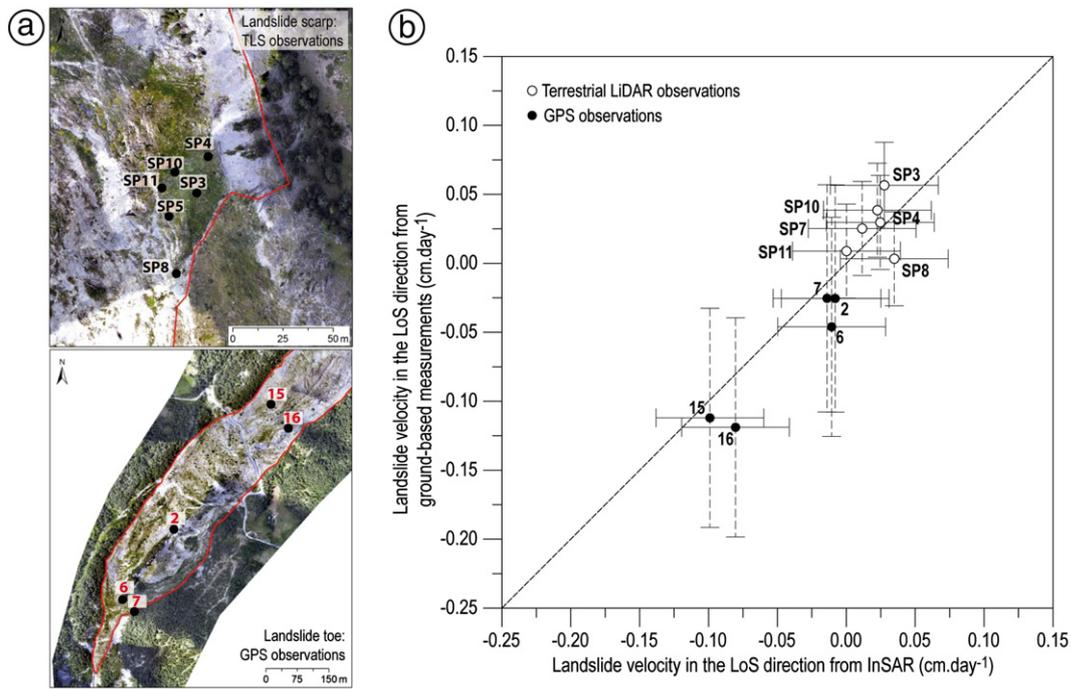
**Fig. 8.** Landslide velocity (vertical component and LoS direction) measured by InSAR and ground-based techniques (terrestrial LiDAR in the ablation zone and GPS in the accumulation zone) at La Valette for the period July–October 2009. The uncertainties of each measurement techniques are  $\pm 0.9$  cm for InSAR,  $\pm 7$  cm for GNSS, and  $\pm 3$  cm for terrestrial LiDAR.
