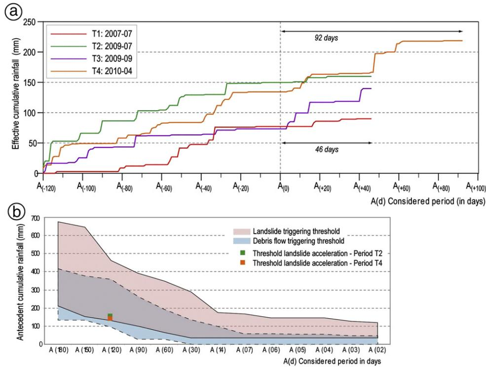
**Fig. 15.** Effect of rainfall amount on landslide motion. Cumulative effective rainfall observed before and during the four InSAR monitoring periods T1 to T4. The rainfall amounts are sampled at the Barcelonnette meteorological station; (b) landslide triggering rainfall thresholds estimated for the Barcelonnette region and threshold for landslide acceleration identified for two InSAR monitoring periods (T2, T4).
