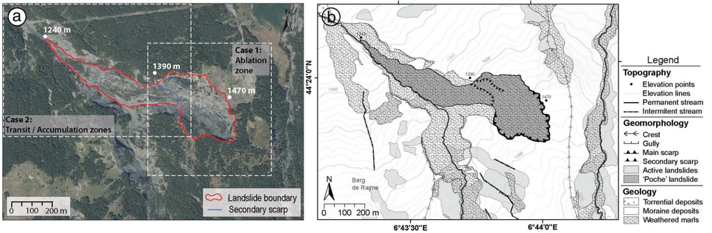
**Fig. 3.** Morphology of the Poche landslide. (a) Orthophotograph of the landslide in 2009 and location of ablation (case 1) and transit-accumulation zones (case 2); (b) morpho-structural map of the landslide.
