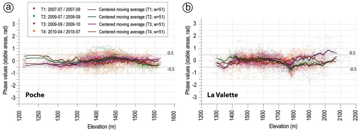
**Fig. 7.** Variability of phase values with elevation. (a) Phase values for the Poche landslide with respectively 83%, 85%, 96% and 64% of values in the range  $\pm 0.5$  rad for the periods T1, T2, T3 and T4. (b) Phase values for the La Valette landslide with respectively 76%, 81%, 80% and 72% of values in the range  $\pm 0.5$  rad for the periods T1, T2, T3 and T4. The centred moving average is calculated for each period with a season  $w = 51$ .
