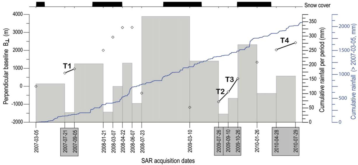
**Fig. 6.** Time acquisition and perpendicular baseline (white point) of the SAR images together with the cumulative net rainfall between consecutive SAR acquisitions (grey box) and for the complete time period (blue line) at the Barcelonnette meteorological station. The presence of snow cover (black box) is estimated from satellite image analysis. The interferograms T1, T2, T3 and T4, analysed in this work, are indicated.
